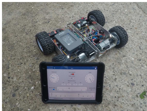
Fig. 14. The completed robotic car controlled by a tablet
