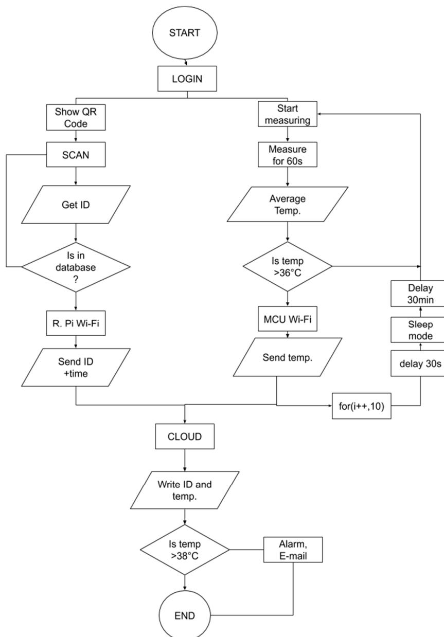
Fig. 4. Functional principle of the proposed system
