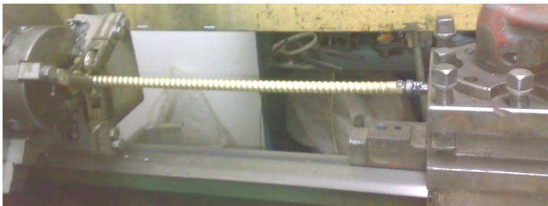
*Fig. 3. The process of manufacturing a spiral corrugated tube by the method of roller spinning on the 16K20 screw lathe [4]*
