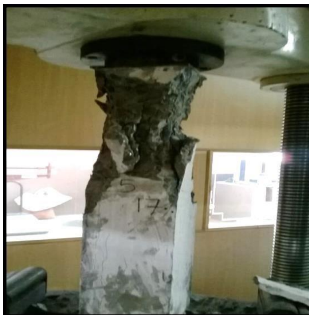
Fig. 5. Failure pattern of a concrete column with a 100% of OPC [38]
