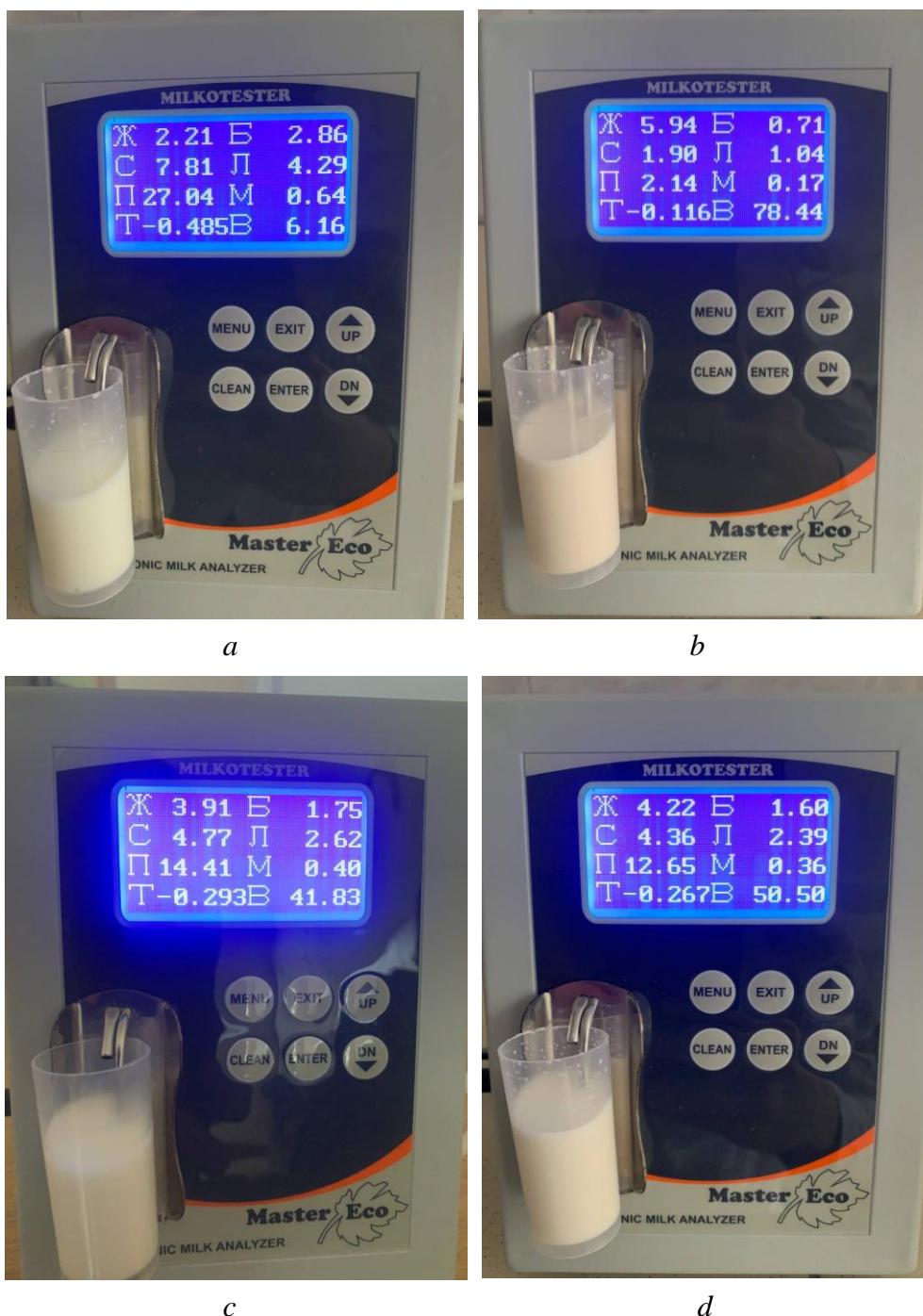
Fig. 1. Photo of the results of the analysis of cow 's milk (a), nut milk (b), a 50:50% mixture (c), a mixture of 60% nut milk and 40% cow 's milk (d):
