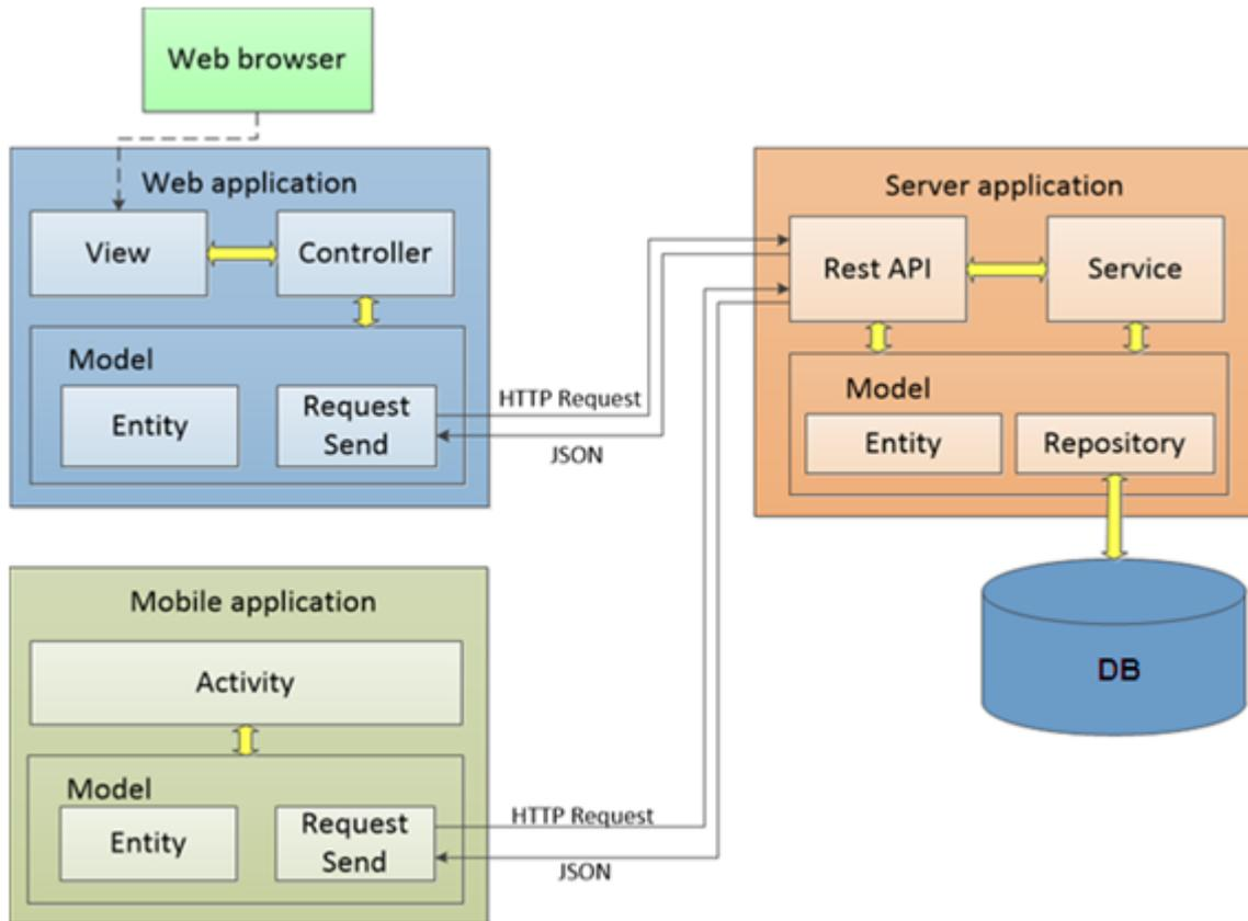
Fig. 2. The structure of the software subsystem
