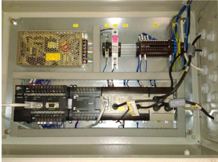
Fig. 3. Control unit of camera system F150-C10E-3
