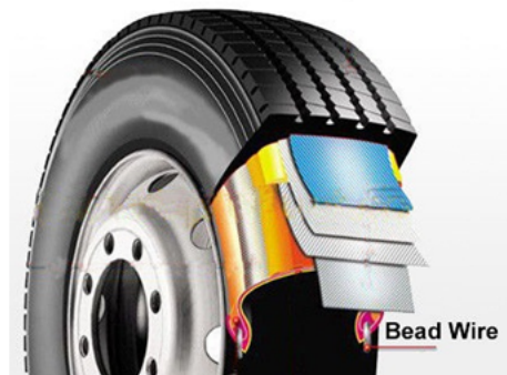
Fig. 1. The bead wire and its placement
