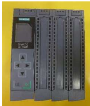
Fig. 12. PLC SIEMENS Simatic S7-1500 CPU 1512C-1PN
