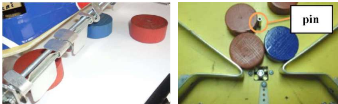
Fig. 4. Puck collector and sorting place in undercarriage of the robot
