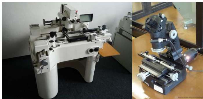
Fig. 1. Example of Laboratory measuring microscope (left) and example of Toolmakers microscope (right)
