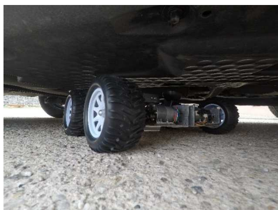
Fig. 15. Final robotic car during chassis inspection
