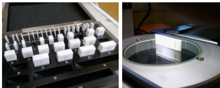
Fig. 8. Length gauge blocks
