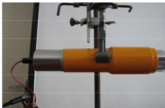
Fig. 6. Model of design of collimator and laser diode
