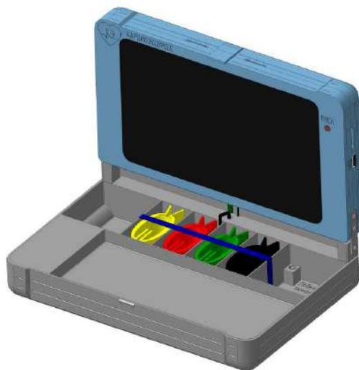
Fig. 4. The portable electrocardiograph: 3D-model
