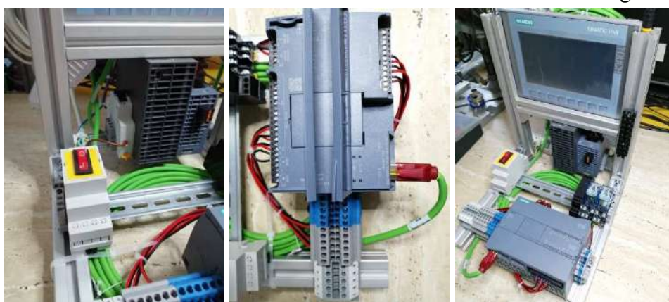
Fig. 7. Total red highlighted power switch (left); additional screw terminal (middle); Profinet switch (right)
