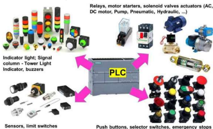
Fig. 1. Concept of controlled system including the PLC controller
