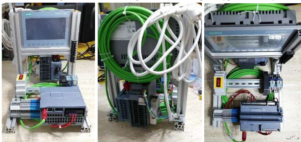
Fig. 6. Training PLC stand overall configuration (left); back side of stand with power supply and circuit breaker (middle); upper view to stand (right)
