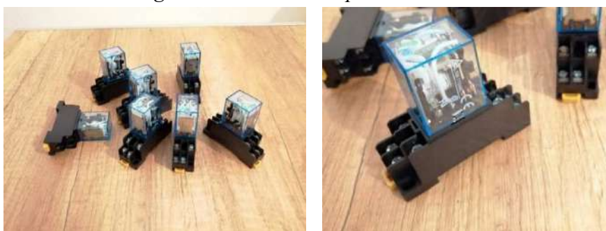
Fig. 6. Relay mounted on pluggable DIN socket
