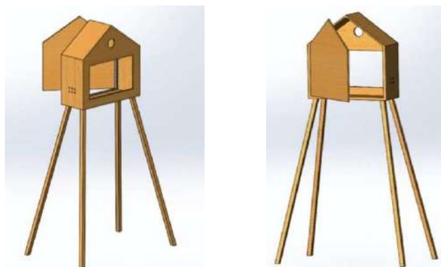
Fig. 6. Design of the case of the photo booth: front and back view
