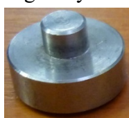
Fig. 1. Reference object for CoG determination
