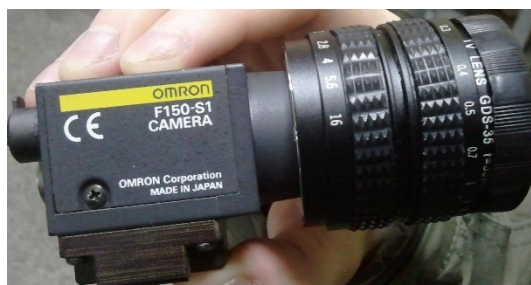
Fig. 4. Camera F150-S1 with 35mm CCTV lens
