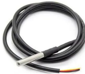
Fig. 4. Temperature sensor DS18B20 [14]
