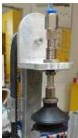
Fig. 8. Bag suction cup with a spring holder
