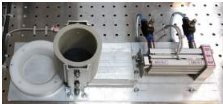
Fig. 6. Gravity tank of objects with feeder
