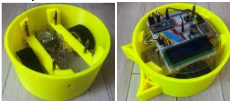
Fig. 7. Connection of the protective frame and the chassis of the robot and the overall implementation of the mechanical part of the robot
