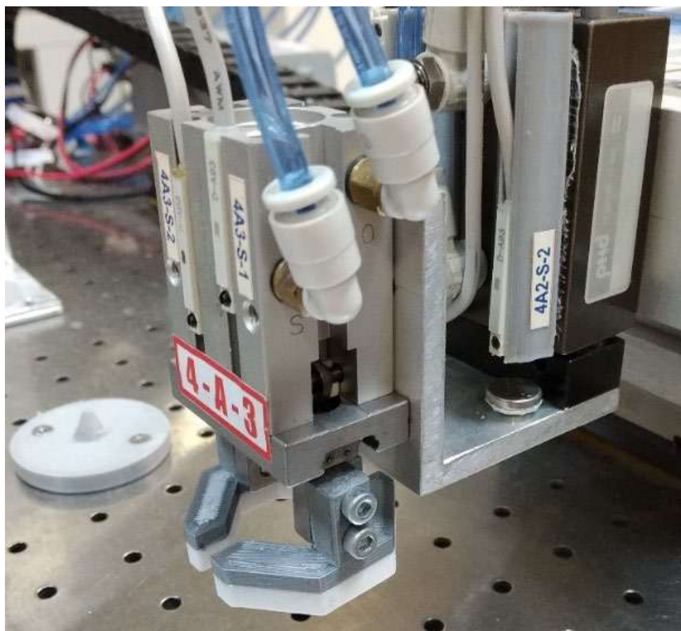
Fig. 10 A view of the grasping effector with 3D printed fingers (4-A-3 gripper).
