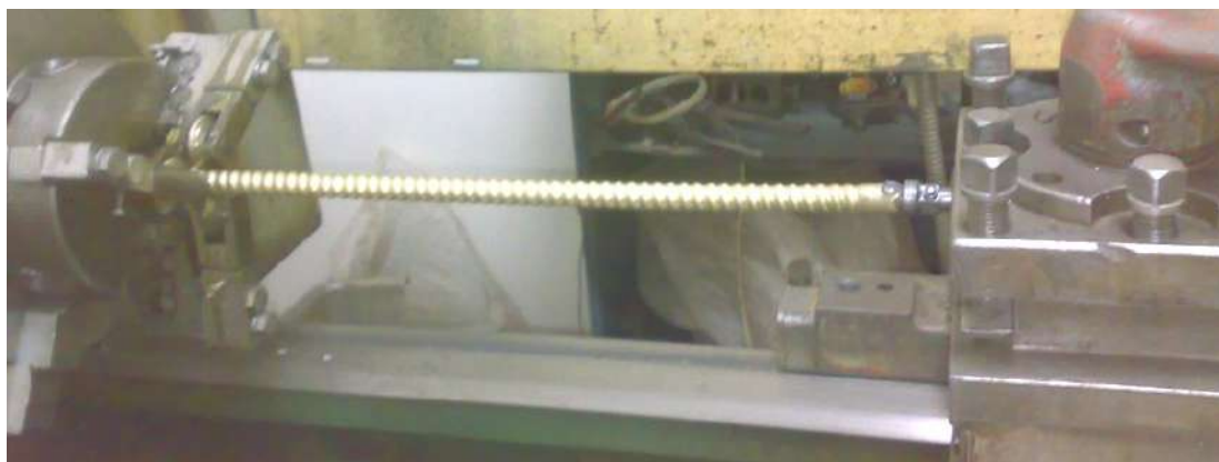
Fig. 3. The process of manufacturing a spiral corrugated tube by the method of roller spinning on the 16K20 screw lathe [4]
