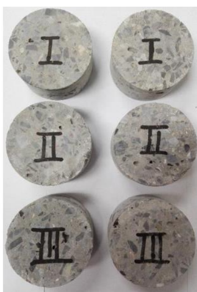
Fig. 3. Images of the series I, II, III (according to Table 3) concrete for quasi-static and dynamic tests [34]
