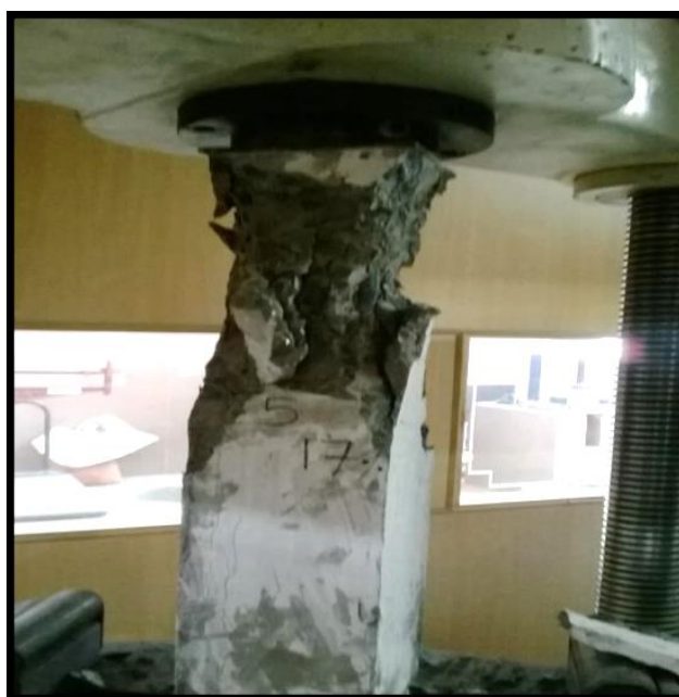
Fig. 5. Failure pattern of a concrete column with a 100% of OPC [38]
