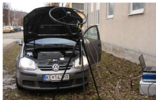
Fig. 6. Location of ring antenna from the engine space
