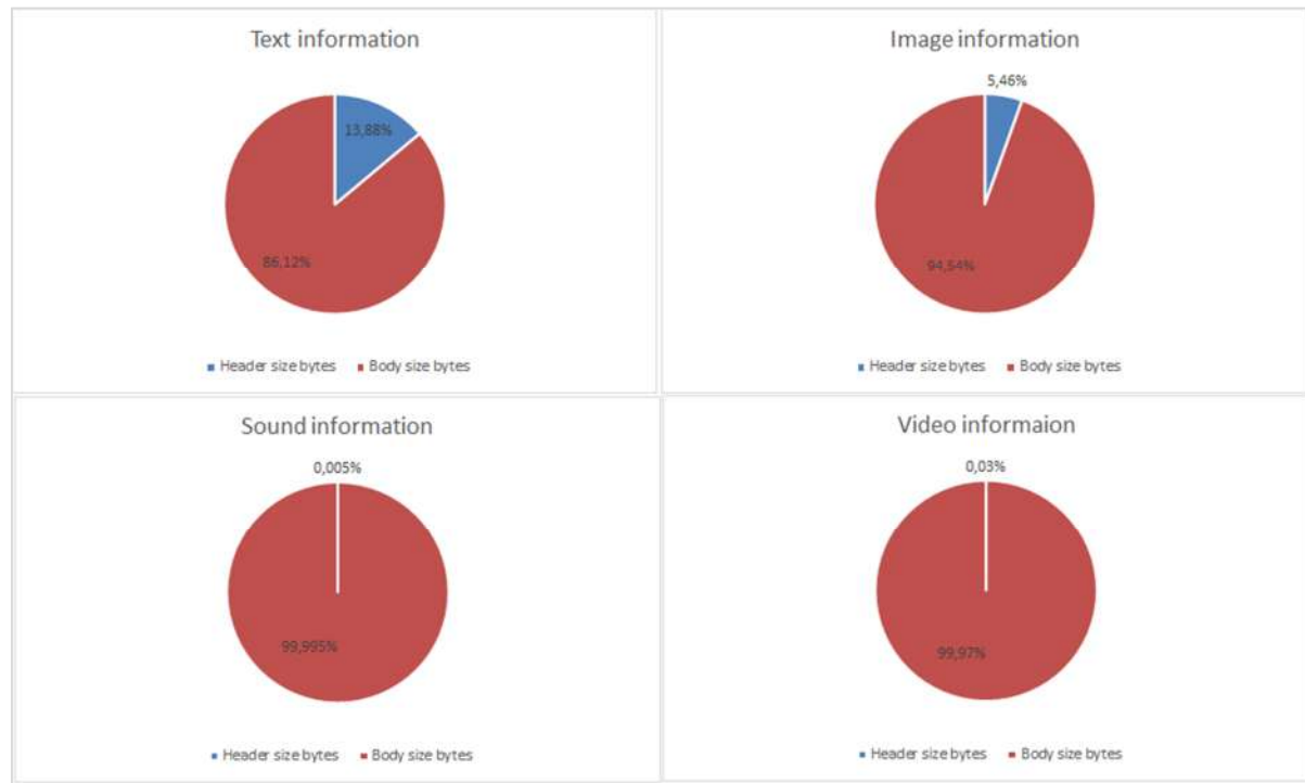
Fig. 4. Ratio of packets' body size to header size by type of information
