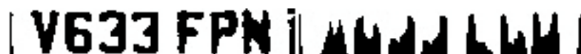
Fig. 3. Binary image of the license plate and the count of white pixels (on Y-axis) by the columns
