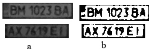
Fig. 2. Source and binarized images of license plates
