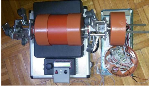
Fig. 2. Wheeled machine with helical motion inside pipe
