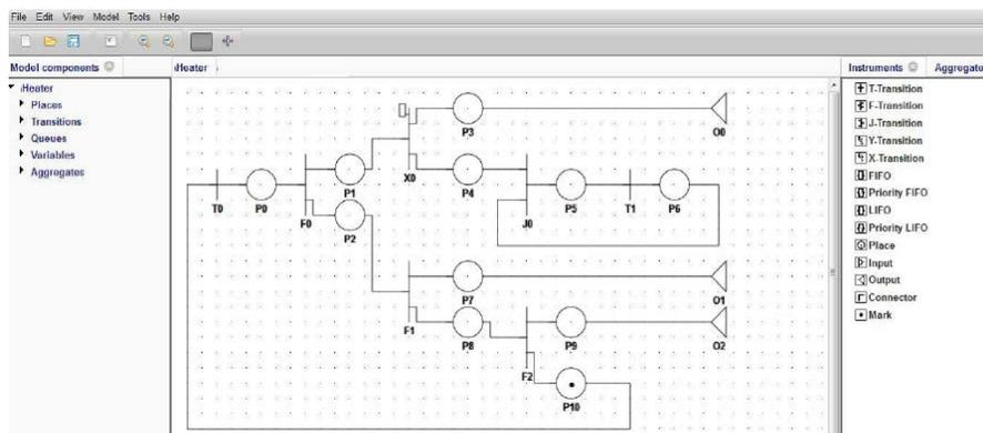
Fig. 6. Plan model in EMS
