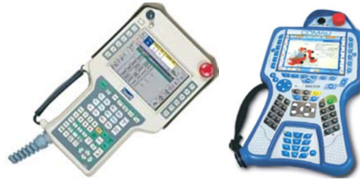
Fig. 2. Programmer OTC Daihen robots and Comau Robotics
