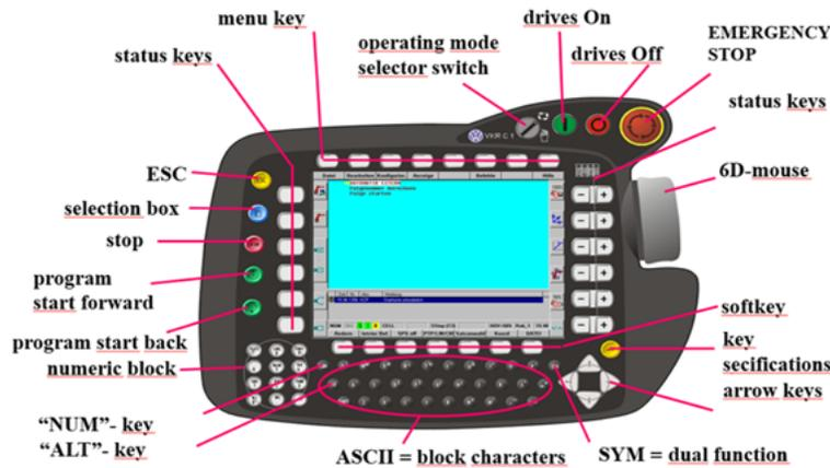
Fig. 4. Programming unit - pendant for robot programming
