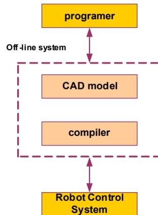
Fig. 5. Procedure for off-line programming of robots
