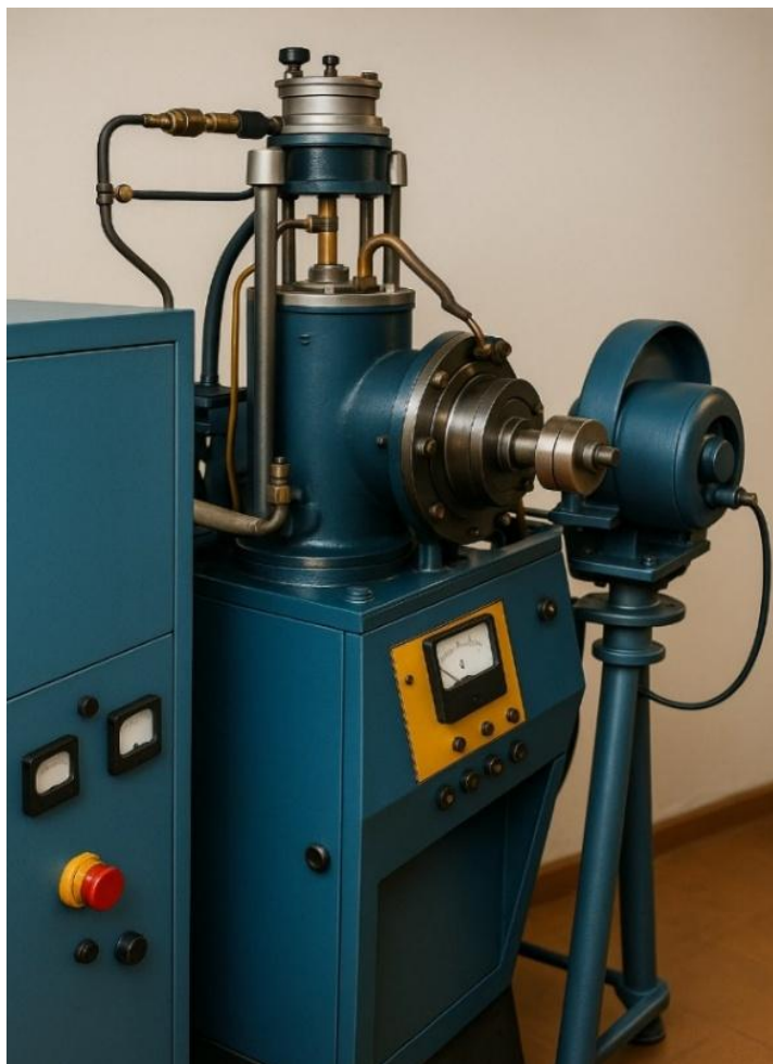
Fig. 6. Diffusion welding setup in a glow discharge equipped with a photoelectric pyrometer PEP-4 [rejuvenated by AI]
