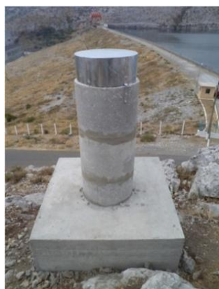
Fig. 2. Appearance of a geodetic pillar for forced centering of instruments
