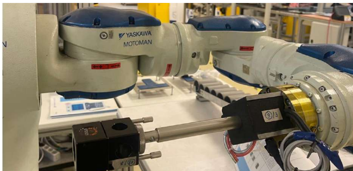
Fig. 2. Reflector mounted on the endpoint of the robot.
